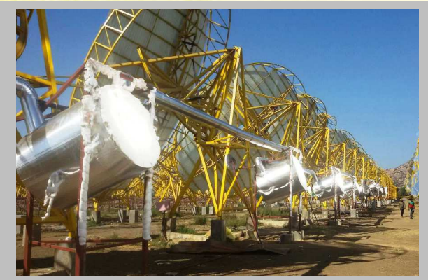
Testing various charging & discharging options of 10 receivers connected in series
